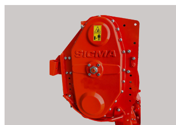
Cast iron cover - strengthens the side transmission
