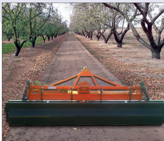
Optional roller cleans, fills and rolls orchard floor
